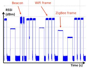
Figure 4. Live capture of RSSI (dBm) measured by the USRP over time.
